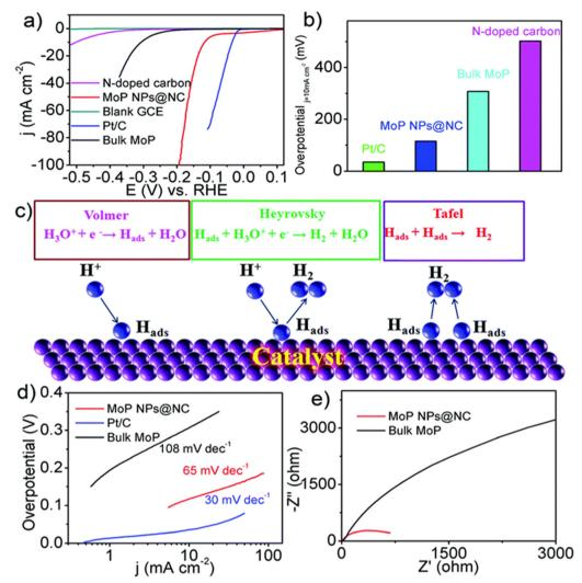
Fig. 13 Polarisation curve (a), the overpotential values at 10 mA cm<sup>-2</sup> (b), the HER (c), Tafel plot (d) and Nyquist plot (e). Reproduced from ref. 118 (Copyrights 2022, Royal Society of Chemistry)
