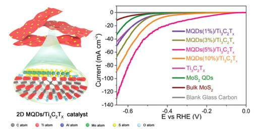
Fig. 8 The overall graphical representation of HER with MoS<sub>2</sub> QDs with MXene composite. Reproduced from ref. 111 (Copyright 2022, The Royal Society).
