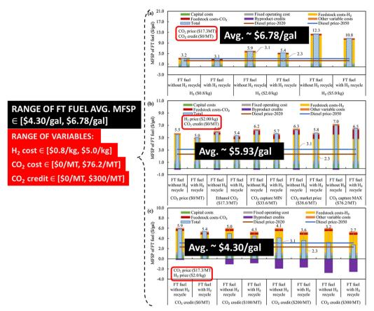
Fig. 17 MFSP of SAF (FT fuel) as a function of the  $H_2$  production cost,  $CO_2$  cost, and the credit for saved carbon for a production capacity of 351 MT per day (divided among 90 MT per day of naphtha, 164 MT per day of jet fuel, and 97 MT per day of diesel). Adapted from ref. 99.
