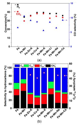
Fig. 16 Catalyst performance for the FT synthesis in terms of (a) the CO<sub>2</sub>/ H<sub>2</sub> conversion rate and (b) selectivity to hydrocarbons, especially longerchain carbons (SAF). From ref. 102.
