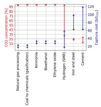
Fig. 7 Range of CO<sub>2</sub> concentration in % (red colored legend) and the corresponding carbon capture costs in \$ per ton of CO<sub>2</sub> captured (blue colored legend) for specific industrial applications. The figure was created using the data from ref. 5.
