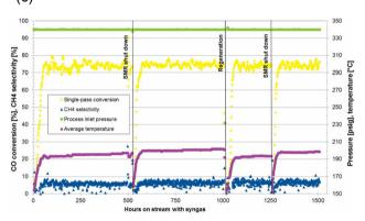
Fig. 23 (a) Velocys' first FT gas-to-liquid technology plant at Oklahoma City, US. From ref. 113. (b) Image of Velocys' FT reactor for the synthesis of hydrocarbons, particularly the SAF. (c)  $\sim$ 1500 hours of operational data from Velocys' synthetic diesel plant. From ref. 113.
