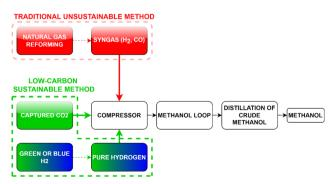
Fig. 8 Block diagram illustrating the traditional and renewable (pure H<sub>2</sub> with captured CO<sub>2</sub>) methods of methanol production. Modified after ref. 76
