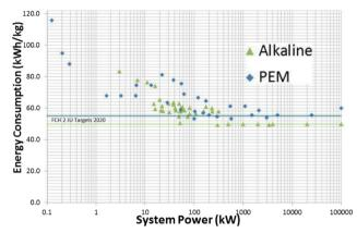
Fig. 6 Electrolysis energy consumption (indicator of efficiency) versus system size of the alkaline (from Pure Energy, McPhy, Hydrogenics, and IHT) and PEM (from Nel, ITM, Hydrogenics, and Areva) electrolyzers for a range of commercially available electrolyzers.51
