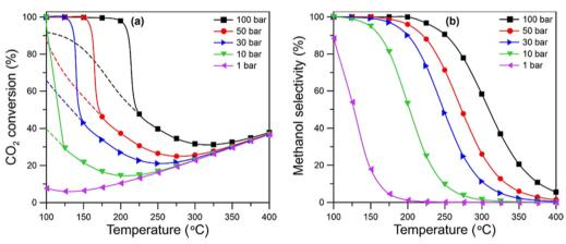
Fig. 10 Sensitivity of methanol synthesis (from CO<sub>2</sub> and H<sub>2</sub>) as a function of pressure and temperature.<sup>77,86</sup>
