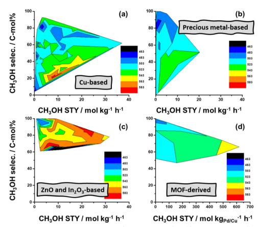
Fig. 11 Contour plots depicting catalytic performance in selectivity (conversion rate; in C-mol%) and space-time yield (STY; production rate; in mol  $kg^{-1}h^{-1}$ ) domain versus the reaction temperature (in K; color legend). The e-methanol production rate with MOF/ZIF-derived catalysts is normalized on active metals. Adapted from ref. 88.
