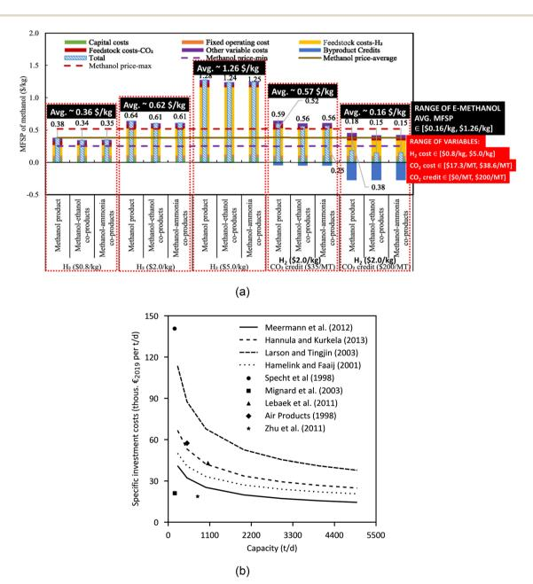
Fig. 13 (a) MFSP of e-methanol as a function of the H<sub>2</sub> production cost, CO<sub>2</sub> cost, and the credit for saved carbon, for a production capacity of 1190 MT per day. Adapted from ref. 78. (b) Cost of e-methanol production versus production plant capacity. From ref. 97.
