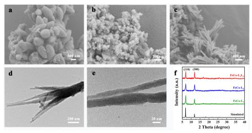
Fig. 1 (a) SEM image of FeCo- $L_1$ , (b) SEM image of FeCo- $L_2$ , (c) SEM images and (d) (e) TEM images of FeCo- $L_1$ L<sub>2</sub>, (f) XRD patterns of the as-synthesized FeCo- $L_1$ , FeCo- $L_2$ , and FeCo- $L_1$ L<sub>2</sub> with the corresponding simulated patterns.
