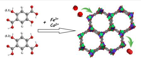
Scheme 1 Schematic illustration of the synthesis of FeCo-L<sub>1</sub>L<sub>2</sub> electrocatalysis.
