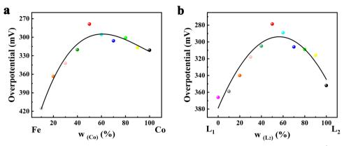
Fig. 4 Volcano-type plots of overpotential with (a) different metal atom ratios and (b) different ligand ratios at 10 mA cm<sup>-2</sup>.
