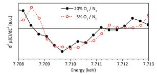
Fig. 9 Analysis of the low intensity peak at  $E < E_0$  in the Co-K edge XANES of LSC at 700 °C under synthetic air and 5% O<sub>2</sub>/N<sub>2</sub>
