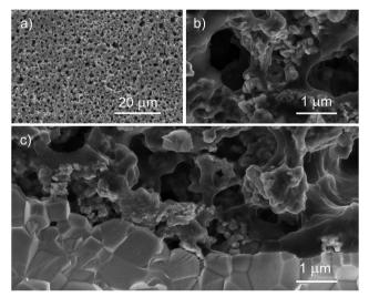
Fig. 1 SEM micrographs of LSC75–GD $_{\rm CC}$ C25 cathode. (a) Top view at low magnification. (b) Detail of top view. (c) Cross section with SDC electrolyte at the bottom. The smallest particles in the cathode belong to the GDC phase.
