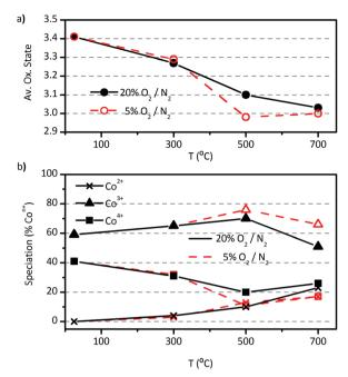
Fig. 8 Analysis of cobalt's oxidation state in LSC nanopowders as function of temperature and under different O2 concentration in the O2/N2 atmosphere. (a) Average oxidation state, and (b) speciation of cobalt atoms in LSC according to Co-K edge XANES analysis using the LCF method.
