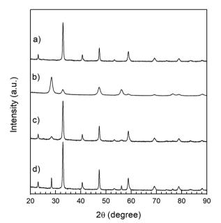
Fig. 3 XRD patterns. (a) LSC nanopowders; (b) GDC powder with particles of spherical shape; (c) LSC75-GDC<sub>MW</sub>25 cathode before the sintering process; (d) LSC75-GDC<sub>MW</sub>25 cathode after 2H at 850 °C.
