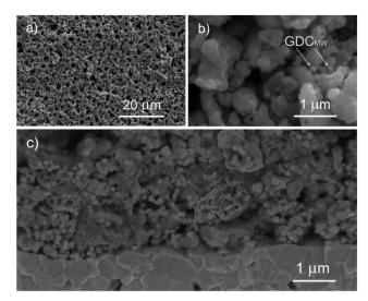
Fig. 2 SEM micrographs of LSC75-GD<sub>MW</sub>25 cathode. (a) Top view (low magnification). (b) Detail of top view. Arrows spot GDC spheres. (c) Cross section including SDC electrolyte. Largest cathode's particles belong to LSC phase.
