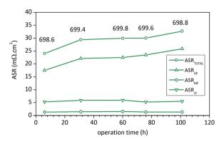
Fig. 7 Long-term operation test of LSC75-GD<sub>MW</sub>25 cathode at 700 °C during 101 h under synthetic air flow. The evolution of each component with time shows the origin of the increment in  ${\sf ASR}_{\sf TOTAL}$  observed during the first hours of operation. The inserted numbers indicate the temperature of the sample in °C when the measurement was performed.
