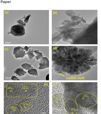
Fig. 4 TEM micrographs of the as-prepared MoO<sub>2</sub> nanoparticles of (a), (b) N1 and (c), (d) M1 samples; HRTEM micrographs of the (e) N1 and (f) M1 samples
