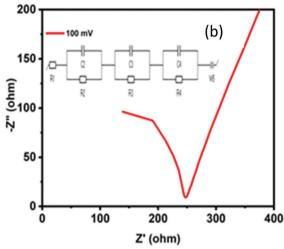
Fig. 6 Nyquist plots (EIS curves) of (a) N1 and (b) M1. The inset figure (a) and (b) represents the equivalent circuit model of the EIS plots fitted by EC lab Z-fit software
