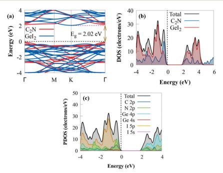
Fig. 3 (a) Projected electronic band structure, (b) DOS and (c) PDOS of the  $Gel_2/C_2N$  vdW heterostructure. The Fermi level is set to zero.
