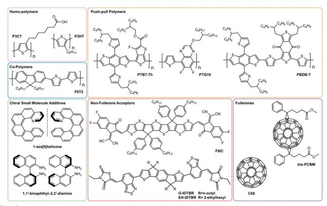
Fig. 1 Summary of the  $\pi$ -conjugated organic semiconducting molecules discussed as part of this review, grouped into homo-polymers, co-polymers, chiral small molecule additives, push-pull polymers, non-fullerene acceptors and fullerenes.
