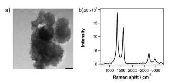
Fig. 1 (a) TEM image of dahlia-shaped SWCNH bundles. Scale bar is 50 nm. (b) Raman spectra of SWCNHs, excited with a 532 nm laser.
