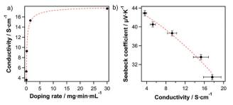
Fig. 3 (a) Conductivity of SWCNHs as a function of OA doping rate. (b) The Seebeck coefficient as a function of conductivity upon OA doping. The lines serve as a guide to the eye.
