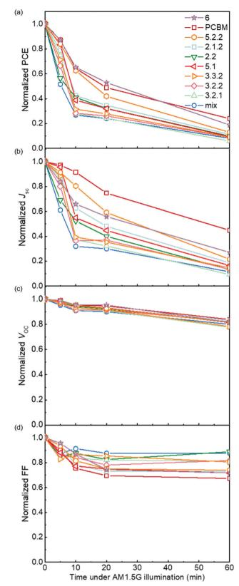
Fig. 3 Photovoltaic parameters (a) power conversion efficiency (PCE), (b) short circuit current density  $J_{\rm sc}$ , (c) open circuit voltage  $V_{\rm oc}$  and (d) fill factor FF of PCDTBT:fullerene devices as a function of the time for which the active layer had been exposed to simulated AM 1.5G illumination in air prior to electrode deposition. All performace parameters are normalised to the value measured for a device whose active layer was not exposed to air.
