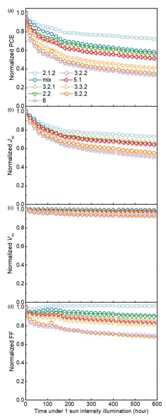
Fig. 5 Evolution of normalised device parameters of the PCDTBT:bis-PCBM devices under continuous 1 sun intensity illumination in a nitrogen atmosphere. All parameters are normalised to their initial performance.
