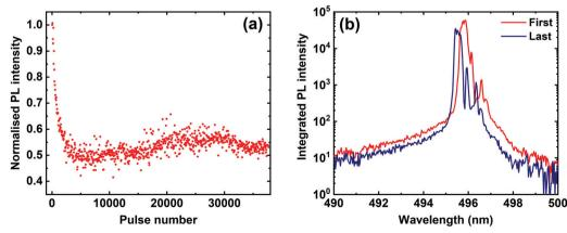
Fig. 4 Above threshold photostability data. Part (a) shows the integrated intensity versus number of pulses for the DPAVB/PS cavity at  $P = 2 P_{th}$ . Part (b) shows the first (red) and last (blue) spectra recorded, indicating that the microcavity remained in the non-linear emission regime over more than 37 000 pulses.
