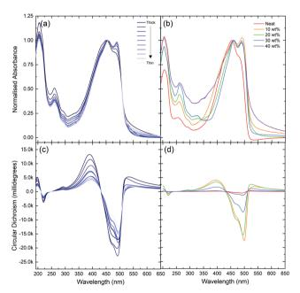
(a and b) Absorption and (c and d) circular dichroism spectra for (a and d) F8T2:10 wt% [M]-aza[6]H blends as a function of film thickness and (b and d) 100 nm thick F8T2: [M]-aza[6]H blends as a function of aza[6]H loading ratio.
