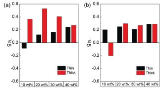
Fig. 3 (a)  $g_{\rm PL}$  and (b)  $g_{\rm EL}$  of thin ( $\sim$ 60 nm) and thick ( $\sim$ 100 nm) F8T2: [P]-aza[6]H films and devices
