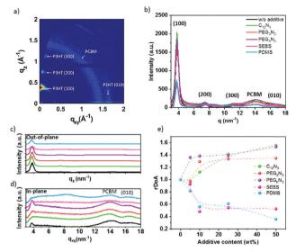
Fig. 4 (a) Two-dimensional GIWAXS image of P3HT:PC<sub>61</sub>BM thin film (b) Effect of the additives on 2D GIWAXS diffraction pattern: (b) fully integrated, (c) out-of-plane integrated and (d) in-plane integrated signal, and (e) the relative degree of aggregation to neat P3HT:PC<sub>61</sub>BM of (100) peak.
