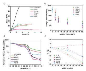
Fig. 5 Effect of the additives on the mechanical properties i.e. (a) stressstrain curves with 50 wt% additive content. (b) Average Young's modulus according to the weight percent of additives added into P3HT:PC61BM blend prior to annealing. (c) Temperature dependence of storage modulus for the P3HT: PC61BM: additive composites (1:0.8:0.4), i.e., in the presence of 50 wt% additives. (d) Summary of the alpha temperature.
