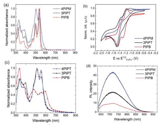
Fig. 3 (a) Normalized optical absorption of  $5 \times 10^{-6}$  M solutions in chloroform, (b) cyclic voltammograms measured in dichloromethane, (c) normalized solid state UV-Vis absorption spectra and (d) photoluminescence spectra of PIPB (red), 3PIPT (black) and 4PIPM (blue) films.
