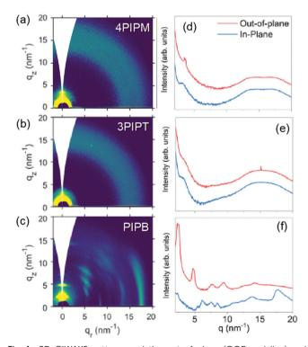
**Fig. 4** 2D GIWAXS patterns and the out-of-plane (OOP, red line) and in-plane (IP, blue line) cuts of the corresponding 2D-GIWAXS patterns of the three acceptors **4PIPM** (a and d), **3PIPT** (b and e) and **PIPB** (c and f).
