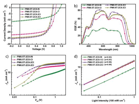
Fig. 2 (a) J-V curves of PM6:5T-2C8-IN/5T-2C8-1Cl/5T-2C8-2Cl and PM6:6T-2C8-2Cl based devices under one sun illumination (AM 1.5G 100 mW cm<sup>-2</sup>). (b) EQE spectra of the corresponding devices. (c)  $J_{ph}$  versus  $V_{eff}$  and (d) light-intensity (P) dependence of  $J_{sc}$  measurement of the devices.
