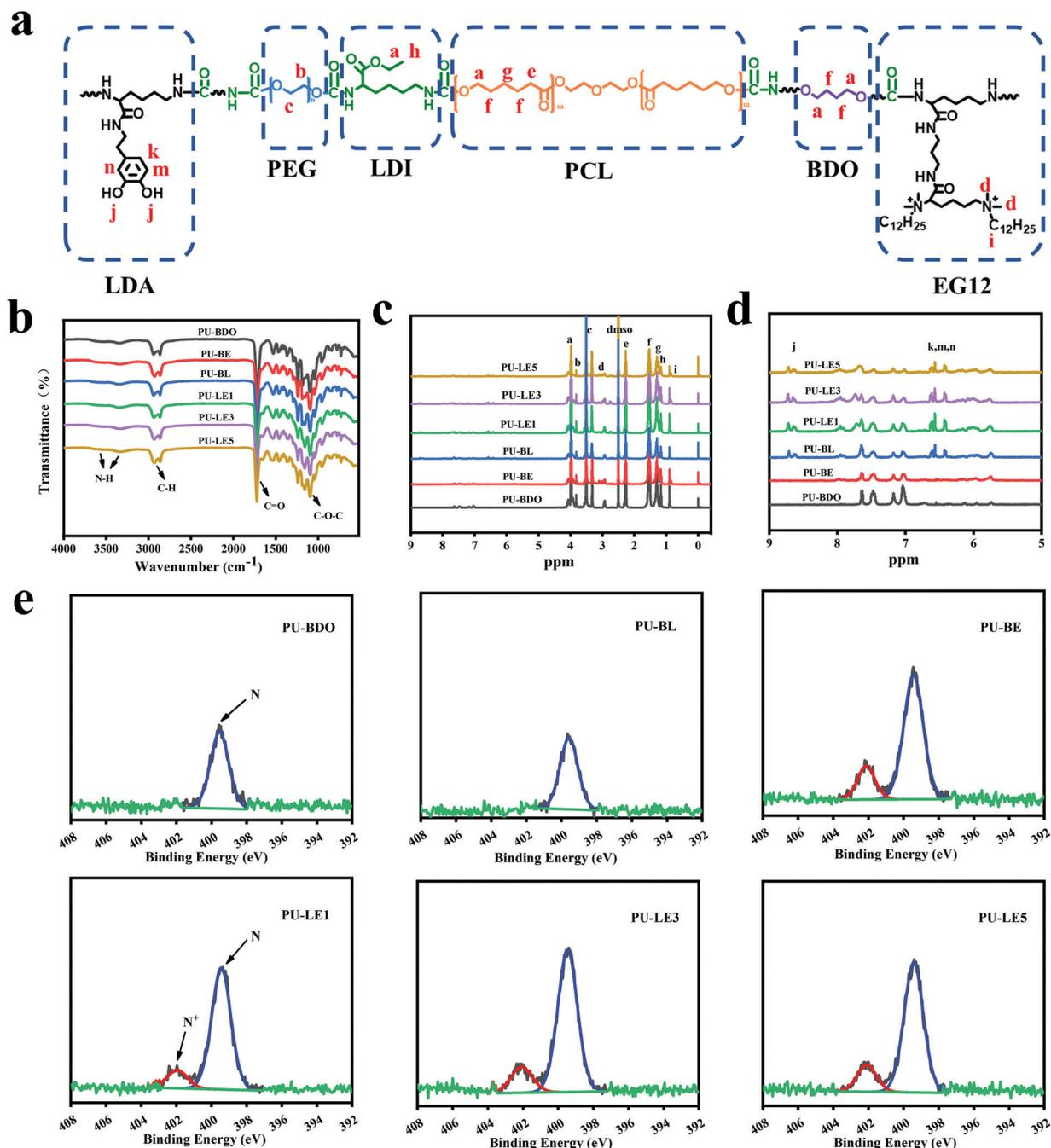
Fig. 2 (a) Structural formula of the representative polyurethane. (b) FTIR spectra of polyurethane membranes. (c)  $^1\text{H}$  NMR spectra of polyurethane membranes. (d) Magnified  $^1\text{H}$  NMR spectra from 5 to 9 ppm. (e) N 1s XPS spectra of polyurethane membranes.
