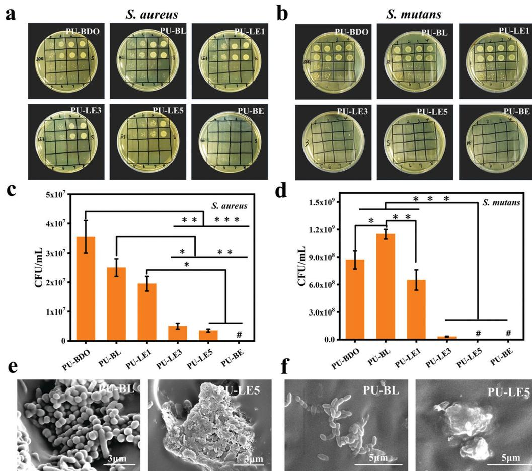
Fig. 6 Colony growth of *S. aureus* (a) and *S. mutans* (b) cultured with polyurethane membranes at different dilutions. The numbers 1–8 represent the samples diluted 10–10<sup>8</sup> times. Quantitative analysis of the colony forming units (CFU) of *S. aureus* (c) and *S. mutans* (d). SEM images of *S. aureus* (e) and *S. mutans* (f) after incubating with PU-BL and PU-LE5 for 24 h. \**P* < 0.05, \*\**P* < 0.01, and \*\*\**P* < 0.001.
