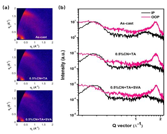
Fig. 4 (a) Two-dimensional GIWAXS scattering patterns and (b) the corresponding profiles for the binary PTQ10:Y26 blend films under different conditions.
