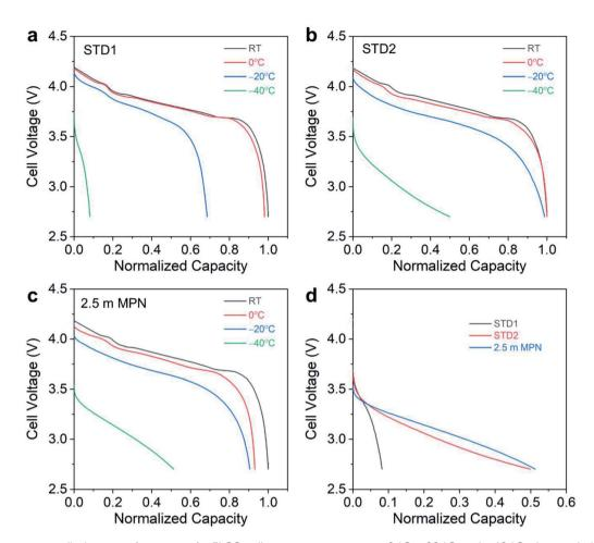
Fig. 6 Low-temperature discharge performance of  $gr\parallel LCO$  cells at room temperature, 0 °C, -20 °C, and -40 °C when cycled in (a) STD1, (b) STD2, and (c) 2.5 m MPN electrolytes. (d) Discharge curves of STD1, STD2, and 2.5 m MPN at -40 °C.
