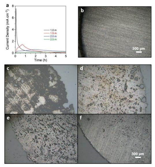
Fig. 1 (a) Chronoamperometry curves with an imposed potential of 4.5 V vs. Li/Li<sup>+</sup> for 5 h of aluminum current collectors when contacting 1.0, 1.5, 2.0, and 2.5 m LiTFSI in MPN electrolytes. Optical micrographs of (b) pristine aluminum, (c) 1.0, (d) 1.5, (e) 2.0, and (f) 2.5 m concentration after corrosion tests.
