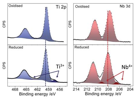
Fig. 3 XPS spectra of oxidised (upper panel) and reduced (lower panel) Nb doped TiO<sub>2</sub> in the Ti 2p and Nb 3d regions.
