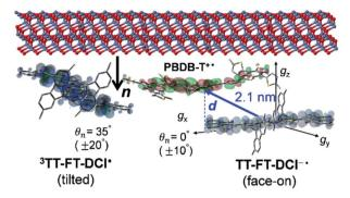
Fig. 13 Molecular orientations of the triplet exciton and the reduced radical in the CS state in the PBDB-T:TT-FT-DCI blend film
