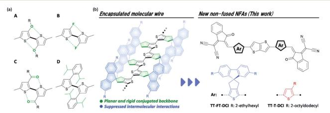
Fig. 1 (a) Typical intramolecular interactions found in non-fused NFAs, (b) chemical structure of encapsulated oligothiophene molecular wire, and non-fused NFAs developed in this study.
