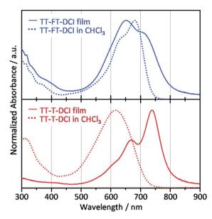
Fig. 5 UV-vis absorption spectra of films (solid lines) and in CHCl<sub>3</sub> solutions (dotted lines) for TT-FT-DCI and TT-T-DCI.
