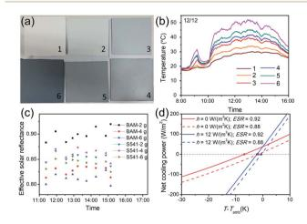
Fig. 4 (a) Optical images of six reference coatings without phosphors. (b) Field test results of the six reference coatings on December 12. (c) Fitted ESR for six fluorescent cooling coatings at noon time. (d) Calculated net cooling power for coatings with different ESR values and non-radiative heat transfer coefficients h. The solar intensity, downward longwave radiation and coating emissivity for modelling were kept as 700 W m $^{-2}$ , 360 W m $^{-2}$  and 0.95, respectively.
