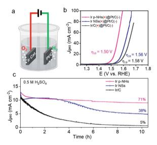
Fig. 4 Initial electrocatalytic overall water splitting performance in 0.5 M  $\rm H_2SO_4$ . (a) Scheme of the two-electrode cell electrolyzer using the Ir-based catalyst as the anode and 20% Pt/C as the cathode. (b) Polarization curves of Ir p-NHs, Ir NSs and Ir/C for overall water splitting. (c) Durability test for the three catalysts in a two-electrode configuration.
