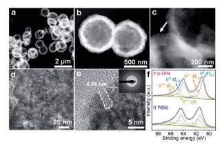
Fig. 2 Structural characterization of Ir p-HNs. (a–c) HAADF-STEM images, (d and e) HRTEM images and the inserted SAED pattern, and (f) high-resolution XPS Ir 4f spectra of Ir p-HNs and Ir NSs.
