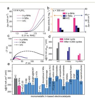
Fig. 3 (a) Polarization curves of the OER, with currents being normalized to geometric surface areas, (b) mass activities and current densities at an overpotential of 300 mV, (c) electrochemical impedance spectroscopy, and (d) overpotentials at 10 mA cm<sub>aeo</sub><sup>-2</sup> before and after 4000 cycles on Ir p-NHs, Ir NSs and commercial Ir/C catalysts. (e) Activity comparison with recently reported monometallic Irbased electrocatalysts in acidic electrolyte.
