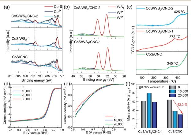
Fig. 3 High-resolution (a) Co 2p and (b) W 4f XPS spectra, and (c) O<sub>2</sub>-TPD profiles of CoS/CNC, CoS/WS<sub>2</sub>/CNC-1, and CoS/WS<sub>2</sub>/CNC-2 catalysts. The polarization curves of CoS/WS<sub>2</sub>/CNC-1 catalyst measured in the (d) RDE and (e) GDE setups during the ADT process, and (f) mass activity ( $J_{\text{mass}}$ ) at 0.80 V versus RHE tested in the GDE configuration.
