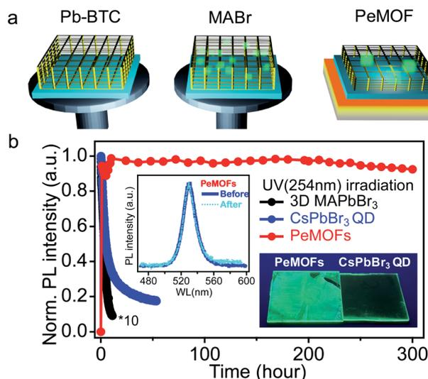
**Fig. 9** (a) Illustration of the PeMOF thin film fabrication process via a two-step spin coating method. (b) Time evolution of the normalized photoluminescence intensities of the 3D MAPbBr<sub>3</sub> thin film, CsPbBr<sub>3</sub> QD thin film and PeMOF thin film. The PL spectrum for a PeMOF thin film before and after UV irradiation is plotted in the inset, and a photo of the PeMOF versus QD thin films after aging is shown in the same plot. Reproduced from ref. 20 with permission.
