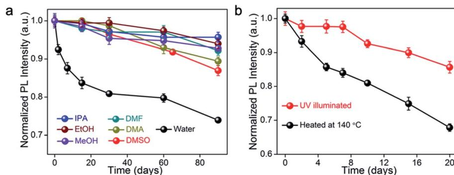
Fig. 6 The normalized PL intensity of the PeMOF fabricated by Mollick *et al.* tested in (a) various solvent systems and (b) over 20 days with heat stress and under constant UV illumination. Reprinted with permission from ref. 103. Copyright 2019 American Chemical Society.
