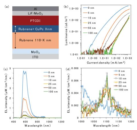
Fig. 2 (a) Schematic of the device with the CuPc-doped rubrene layer at the D/A interface. (b) L-J curves and (c and d) EL emission spectra with a constant current flow (1000 mA cm<sup>-2</sup>) for the devices with 0 nm (blue), 5 nm (orange), 10 nm (grey), 25 nm (yellow), 50 nm (brown), and 100 nm (green) of CuPc-doped rubrene layers at the D/A interface.
