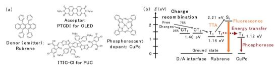
Fig. 1 (a) Chemical structures of rubrene, PTCDI, ITIC-Cl and CuPc. (b) The energy levels of excited states and schematic of the energy transfer inside the device
