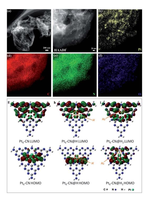
Fig. 2 Morphology and electronic structures of platinum-deposited carbon nitride (Pt/g-C<sub>3</sub>N<sub>4</sub>). (a) STEM image with a scale bar of 200 nm. (b)  $HAADF-STEM\ image\ at\ large\ magnification.\ Elementary\ mappings\ for\ Pt\ (c),\ C\ (d),\ N\ (e),\ and\ O\ (f).\ (g-i)\ Frontier\ molecular\ orbital\ (HOMO-LUMO)$ of N-bonded Pt<sub>6</sub> cluster site for H<sub>2</sub> evolution.
