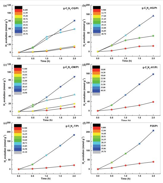
Fig. 3 The general phenomenon for STAP  $H_2$  evolution kinetics. The  $H_2$  evolution yield correlated with system temperature elevation at a variable time under simulated solar light irradiation for the photocatalyst of (a)  $g-C_3N_4-CQ/Pt$ , (b)  $g-C_3N_4-HG/Pt$ , (c)  $g-C_3N_4-HG/Pt$ , (d)  $g-C_3N_4-HI/Pt$ , (e)  $g-C_3N_4-T/Pt$ , (f) P25 (TiO<sub>2</sub>)/Pt. Inset: color scale bar representing system temperature elevation. Photocatalyst loading, 10 mg.
