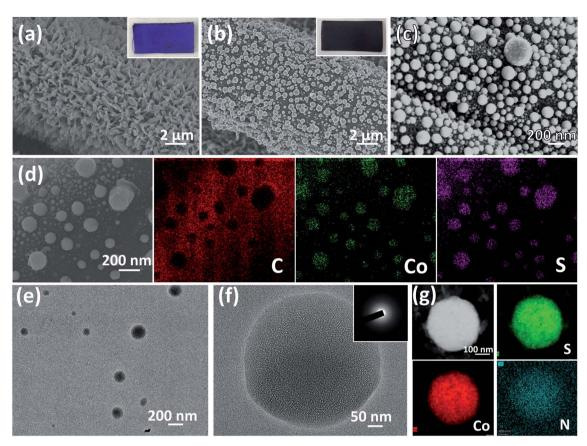
Fig. 1 SEM images of Co-MOF/CC (a) and CoS<sub>x</sub>/CC-L (b and c). Insets are the corresponding photographs. (d) Corresponding EDS mapping of the C element, Co element and S element for  $CoS_x/CC-L$ . TEM (e) and HRTEM (f) images of  $CoS_x/CC-L$ . The inset in (f) is the SAED pattern of CoS<sub>x</sub>/CC-L. (g) Elemental mapping of CoS<sub>x</sub> nanospheres.
