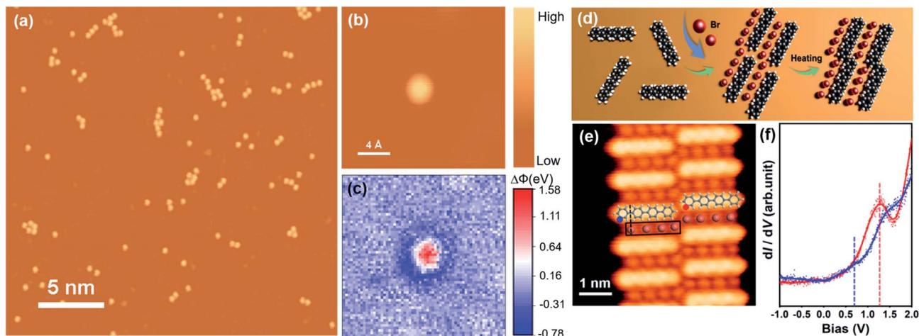
Fig. 5 (a) STM image of highly monodispersed Br atoms on Cu(111). (b) STM image of a single Br atom and (c) its corresponding  $\Delta\phi$  mapping. (d) A schematic process of the coupling reaction mediated by the Br atoms. (e) High-resolution STM image of co-assembled Br atoms and Ph<sub>4</sub>. (f)  $dI/dV$  spectra sampled at the sites highlighted by the coloured dots in (e). Reproduced with permission (d–f).<sup>119</sup> Copyright 2020, American Chemical Society.
