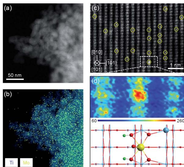
Fig. 2 (a) AC-STEM and (b) EDX mapping images of  $\text{Mo}_1/\text{TiO}_2$ . (c) Atomic-resolution AC-STEM image of  $\text{Mo}_1/\text{TiO}_2$ . (d) Two-dimensional simulated image (above) and the corresponding structural model (below) of the selected area in (c). Light blue represents Ti atoms, red O atoms, green H atoms, and yellow Mo atoms.
