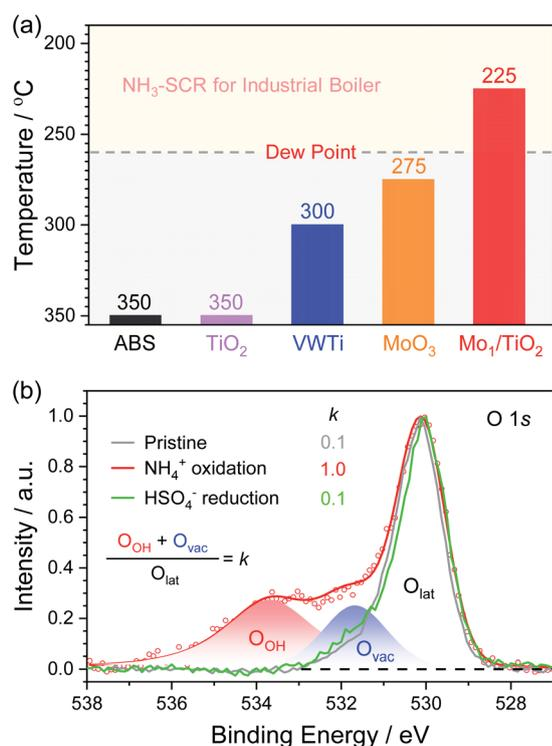
Fig. 6 (a) Onset temperatures of the  $\text{SO}_2$  release over a series of ABS-deposited catalysts. (b) O 1s XPS of  $\text{Mo}_1/\text{TiO}_2$  (pristine and after  $\text{NH}_4^+$  oxidation and  $\text{HSO}_4^-$  reduction).
