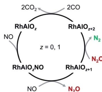
Scheme 1 Proposed catalytic cycle for the conversion of NO and CO into \text{N}_2 and \text{CO}_2 mediated by the neutral \text{RhAlO}_{0-3} species. This catalysis can also be driven by the \text{RhAl}_2\text{O}_{1-4} clusters.
