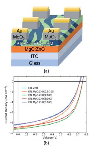
Fig. 1 (a) Schematic of the multi-layered structure of the OPV device. 5 Types of OPVs were tested, 4 with ETLs containing different amounts of Mg-doping in ZnO and an undoped "control" device. (b) Representative current density vs. voltage curves under 1 sun. Corresponding average key performance indicators from 8 distinct devices for each type of ETL are reported in Table 2.
