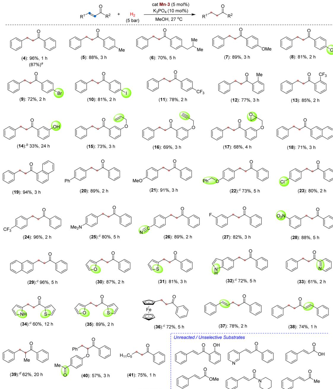
**Scheme 3** Scope of Mn-catalyzed C=C bond hydrogenation of  $\alpha,\beta$ -unsaturated ketones. Reaction conditions: substrate,  $\alpha,\beta$ -unsaturated ketone (0.20 mmol), Mn-3 (0.005 g, 0.01 mmol, 5 mol%),  $K_3PO_4$  (0.0043 g, 0.02 mmol), MeOH (1.0 mL),  $H_2$  (5 bar). Yields are of isolated compounds. <sup>a</sup>Reaction in 0.5 g scale. <sup>b</sup>Reaction at 50 °C. <sup>c</sup>Mixture of MeOH : DCM (4 : 1) used. <sup>d</sup>Reaction at 10 bar  $H_2$  and 50 °C.
