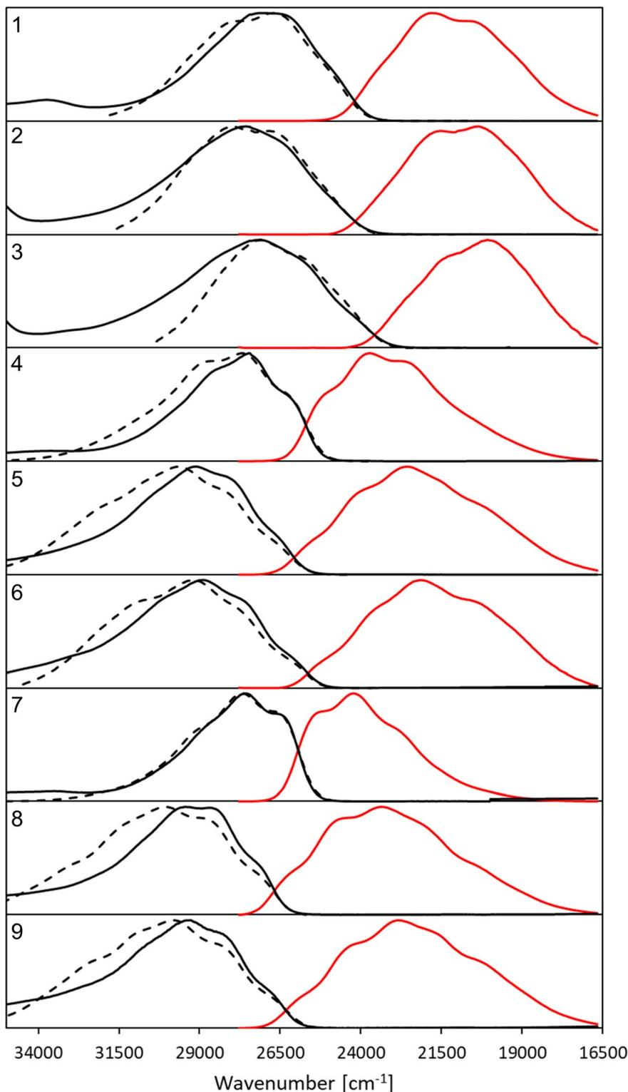
Fig. 2 Normalized, corrected absorption (solid black line), fluorescence (solid red line) and mirror-image of fluorescence spectra (dashed black line) shifted to match the 0–0 point in CHCl<sub>3</sub>.
