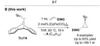
Fig. 1 (A) Organoiron- and fluoride-catalyzed synthesis of phosphiranes by phosphinidene transfer and the proposed intermediate. (B) This work: organoiron-catalyzed phosphinidene transfer to electrondeficient olefins (EWG = electron-withdrawing group).
