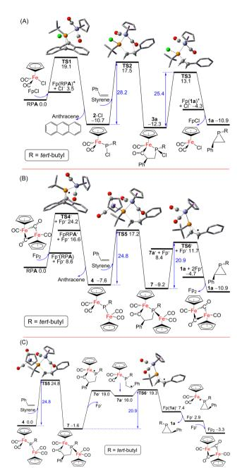
**Fig. 5** DFT computed free energy paths (in kcal  $mol^{-1}$ , at 298 K and 1 M in THF solution) for (A) **2**-Cl (or FpCl) and (B) **4** (or Fp<sub>2</sub>) catalyzed phosphinidene transfer from <sup>1</sup>BuPA to styrene, and (C) the key P–C bond formation steps from **4**. Crucial C, O, P, Cl and Fe atoms in the transition state ball-and-stick models are highlighted as grey, red, orange, green and blue balls, respectively, with most H-atoms omitted for clarity.
