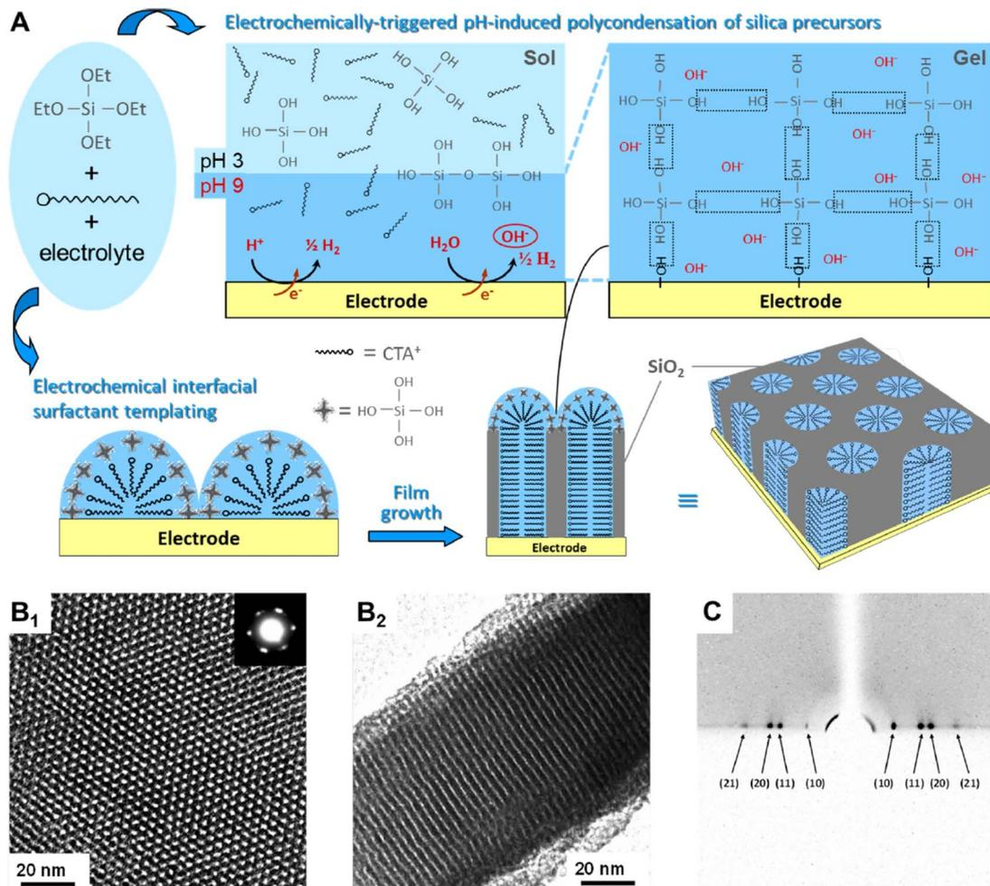
Fig. 3 (A) Schematic illustration of the EASA process. (B) TEM images of the ordered and oriented mesoporous silica film (B<sub>1</sub> top view with electron diffraction pattern as inset; B<sub>2</sub> cross-section). (C) Typical GI-XD pattern confirming the hexagonal packing of vertically aligned mesopore channels. Reproduced with permission from ref. 40.
