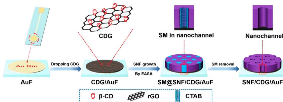
Fig. 12 Illustration of facile preparation of silica nanochannel array film (SNF)/ $\beta$ -cyclodextrin-graphene (CDG)/AuF by EASA method using CDG as nanoadhesive. SM = surfactant micelle. Reproduced with permission from ref. 92.
