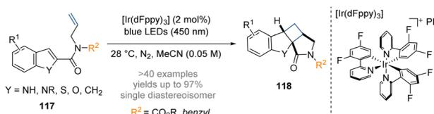
Scheme 34 Dearomative photoredox catalysed intramolecular [2 + 2] cycloaddition of indoles.<sup>40</sup>
