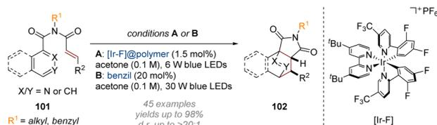
Scheme 29 Dearomative photoredox catalysed intramolecular [4 + 2] cycloaddition of pyridines.<sup>35</sup>
