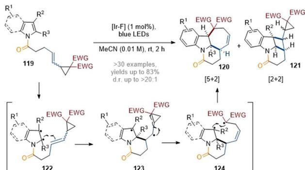
Scheme 35 Dearomatisation of indoles/pyrroles with vinyl-cyclopropanes: synthesis of structurally diverse polycyclic indolines.<sup>41</sup>
