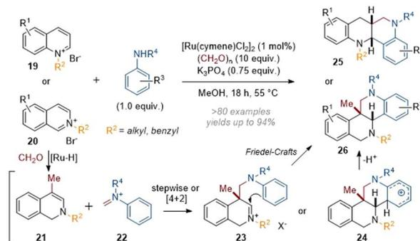
Scheme 7 Mannich-type annulations of activated quinolines and isoquinolines to form polycyclic azaarenes.<sup>12</sup>
