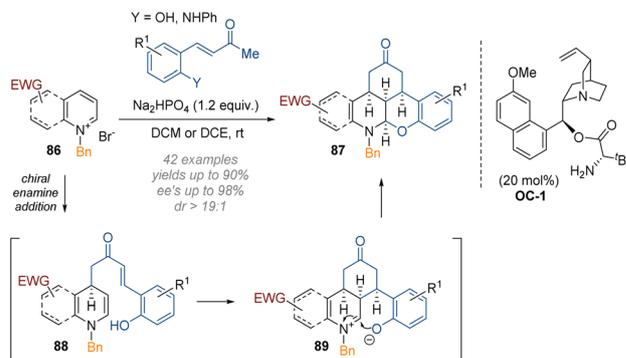
Scheme 25 Enantioselective organocatalytic cascade functionalisation and dearomatisation of pyridinium and quinolinium salts.<sup>31</sup>
