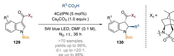
Scheme 38 Organophotocatalytic dearomatisation of indoles, pyrroles and benzo(thio)furans *via* a Giese-type transformation.<sup>44</sup>
