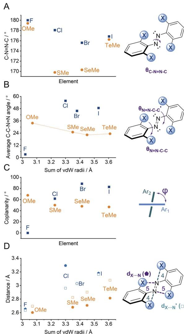
Fig. 5 Geometric parameters from single-crystal data for (*E*)-X<sub>4</sub> (A) C-N=N-C dihedral, (B) average N=N-C-C dihedral, (C) coplanarity of rings, (D) distances between diazo lone pair and X-atom (formation of intramolecular 5 (●) and 4 (□) membered rings).
