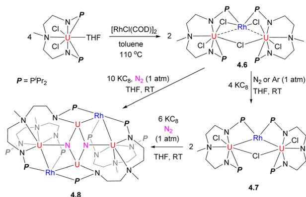
Scheme 35 The synthesis of U/Rh complex and its reactivity in N<sub>2</sub> splitting.
