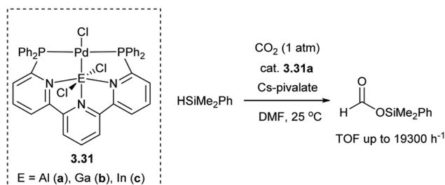
Scheme 26 A series of Pd complexes with “PEP” metalloligands and CO<sub>2</sub> hydrosilylation catalyzed by a Pd(PAIP) complex.
