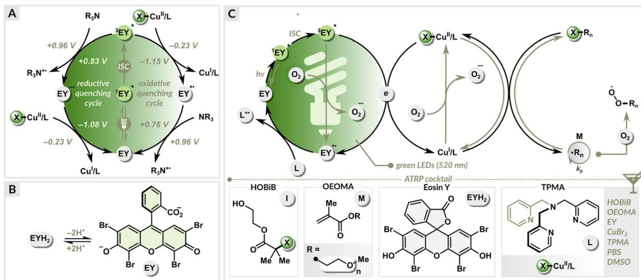
Fig. 2 (A) Reductive quenching vs. oxidative quenching cycle, (B) formation of EY in PBS solution, (C) proposed mechanism.
