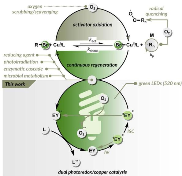
Fig. 1 Approaches for attaining oxygen tolerance in ATRP.
