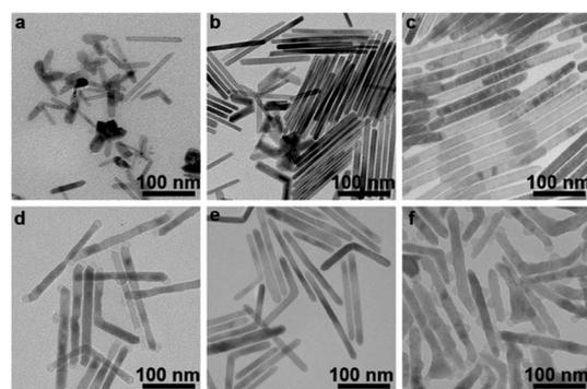
Fig. 2 TEM images of  $\text{CoF}_2$  nanorods: (a) 20 min, (b) 40 min, and (c) 60 min. TEM images of products obtained by injecting solution B (containing different amounts of  $\text{Li}(\text{TFA})$ ) into solution A: (d) 0.05 mmol, (e) 0.01 mmol, and (f) 0.1 mmol.
