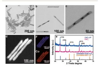
Fig. 1 TEM images of (a)  $CoF_2$  nanorods and (b and c)  $CoF_2$ -LiF heterostructures. (d) Dark field TEM images and the corresponding element mapping spectra of  $CoF_2$ -LiF heterostructures. (e) XRD patterns of  $CoF_2$  nanorods and  $CoF_2$ -LiF heterostructures.
