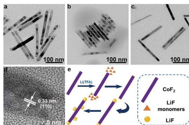
Fig. 3 TEM images of samples after 9 months: (a)  $\text{CoF}_2$ -LiF heterostructures (0.05 mmol), (b)  $\text{CoF}_2$  nanorods, (c)  $\text{CoF}_2$ -LiF heterostructures (0.01 mmol), (d) HR-TEM image of  $\text{CoF}_2$ -LiF heterostructures (0.05 mmol), and (e) schematic of the formation of  $\text{CoF}_2$ -LiF heterostructures.
