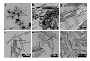
Fig. 2 TEM images of  $CoF_2$  nanorods: (a) 20 min, (b) 40 min, and (c) 60 min. TEM images of products obtained by injecting solution B (containing different amounts of Li(TFA)) into solution A: (d) 0.05 mmol, (e) 0.01 mmol, and (f) 0.1 mmol.
