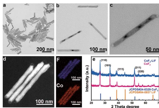
Fig. 1 TEM images of (a)  $\text{CoF}_2$  nanorods and (b and c)  $\text{CoF}_2$ -LiF heterostructures. (d) Dark field TEM images and the corresponding element mapping spectra of  $\text{CoF}_2$ -LiF heterostructures. (e) XRD patterns of  $\text{CoF}_2$  nanorods and  $\text{CoF}_2$ -LiF heterostructures.
