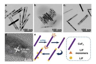
Fig. 3 TEM images of samples after 9 months: (a)  $CoF_2$ -LiF heterostructures (0.05 mmol), (b)  $CoF_2$  nanorods, (c)  $CoF_2$ -LiF heterostructures (0.01 mmol), (d) HR-TEM image of  $CoF_2$ -LiF heterostructures (0.05 mmol), and (e) schematic of the formation of  $CoF_2$ -LiF heterostructures.
