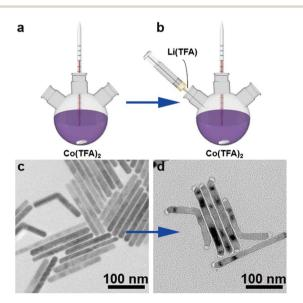
Scheme 1 Schematic of the synthesis of  $CoF_2$  nanorods and  $CoF_2$ -LiF heterostructures.
