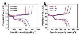
Fig. 5 Galvanostatic charge/discharge curves at 0.1 C rate of (a) CoF2-LiF and (b) CoF2
