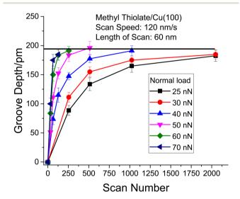
Fig. 3 Plot of the depth of the wear track as a function of the number of passes over a methyl thiolate saturated Cu(100) surface showing an exponential increase in the depth of the wear track, indicative of first-order reaction kinetics. The maximum depth for all mechanochemical reactions is  $\sim\!195$  pm, which agrees well with the calculated thickness of a methyl thiolate films.
