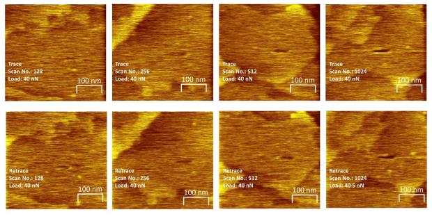
Fig. 2 Low-load AFM images of methyl-thiolate-covered Cu(100) after having been scanned various times in the forward (top traces) and the reverse (bottom traces) direction at a load of 40 nN, where the scan times are shown marked on each image.
