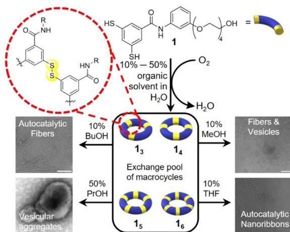
**Scheme 1** Polymorphs emerging from a single building block dynamic combinatorial library (DCL). Building block **1** is oxidised by air to form a DCL of macrocycles that form various polymorphic structures depending on the co-solvent present. Scale bars = 200 nm.
