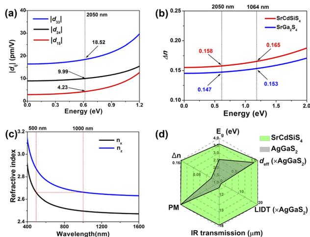
Fig. 6 (a) Frequency-dependent SHG coefficients of  $\text{SrCdSiS}_4$ ; (b) curves of the calculated  $\Delta n$  as a function of energy (eV) for  $\text{SrGa}_2\text{S}_4$  and  $\text{SrCdSiS}_4$ ; (c) calculated refractive index dispersion curves with the shortest PM cut-off edge at 500 nm; (d) radar chart with six directions (representing  $E_g$ ,  $d_{\text{eff}}$ , LIDT, IR transmission, PM,  $\Delta n$ ) to characterize comprehensive IR-NLO performance of  $\text{SrCdSiS}_4$ .
