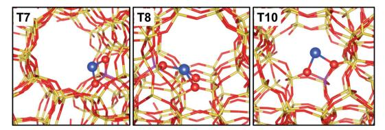
Fig. 3 Graphical representation of Cu<sup>+</sup> sites balancing Al sitting in the T7, T8 and T10 crystallographic positions of ZSM-5. Colour code: blue, Cu; yellow, Si; magenta, Al; red, O. Unpublished figure, structural models obtained from DFT calculations as reported in ref. 37.
