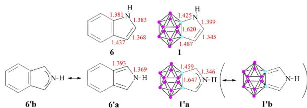
**Scheme 3** Selected bond lengths (in Å) for the pyrrole derivatives (B3LYP/6-311+G\*\*). The elongated C<sub>c</sub>-C bond lengths in **1'** demonstrates the low contribution of the **1'b** resonance structure.
