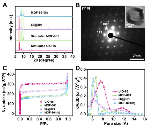
Fig. 2 (A) PXRD patterns of 66@801, MOF-801(h), simulated MOF-801 and UiO-66. (B) SAED pattern of a MOF-801(h) particle (TEM image is shown in the inset). (C)  $N_2$  adsorption–desorption isotherms at 77 K for UiO-66, MOF-801, 66@801 and MOF-801(h). (D) Pore size distribution profiles of UiO-66, MOF-801, 66@801 and MOF-801(h).
