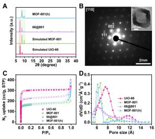
Fig. 2 (A) PXRD patterns of 66@801, MOF-801(h), simulated MOF-801 and UiO-66. (B) SAED pattern of a MOF-801(h) particle (TEM image is shown in the inset). (C)  $N_2$  adsorption—desorption isotherms at 77 K for UiO-66, MOF-801, 66@801 and MOF-801(h). (D) Pore size distribution profiles of UiO-66, MOF-801, 66@801 and MOF-801(h).
