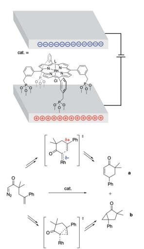
Fig. 4 Parallel electrode plates used to impose external ESFs during the Rh porphyrin-catalyzed rearrangement of 1-diazo-3,3-dimethyl-5-phenylhex-5-en-2-one into products a and b.<sup>26</sup> Key transition states associated with the formation of a and b, which are inequivalently (de) stabilized by the presence of ESFs, are shown.
