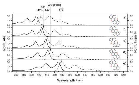
Fig. 5 UV-vis absorption (full line) and emission (dashed line) spectra for N,N-PXX derivatives and PXX in toluene at rt.
