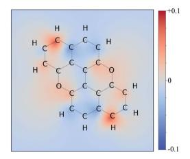
Fig. 3 Excitation charge redistribution map for PXX. This is the excited state CHELPG charges minus ground state CHELPG charges of PXX interpolated over the atomic positions on the  $\sigma$ -scaffold, with the blue and red area indicating the electron depletion and accumulation regions respectively. The colour map ranges from +0.1 (red, donors) to -0.1 (blue, acceptors) electrons.
