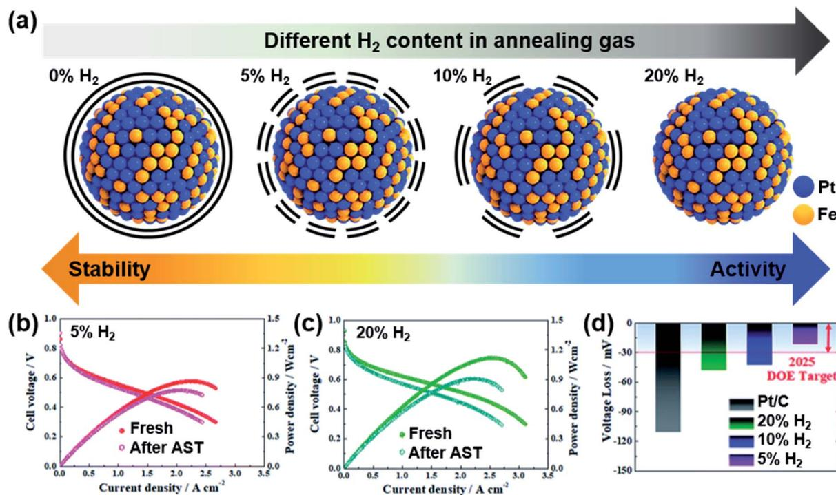
Fig. 5 (a) Difference in the carbon shell depending on annealing conditions; various percentages of H<sub>2</sub> flow were used at 700 °C. *I*-*V* curves before and after accelerated stress tests (ASTs) performed under (b) 5% H<sub>2</sub> and (c) 20% H<sub>2</sub>. (d) Voltage loss at 0.8 A cm<sup>-2</sup> after ASTs. Reproduced from ref. 90 with permission, copyright 2021, the Royal Society of Chemistry.
