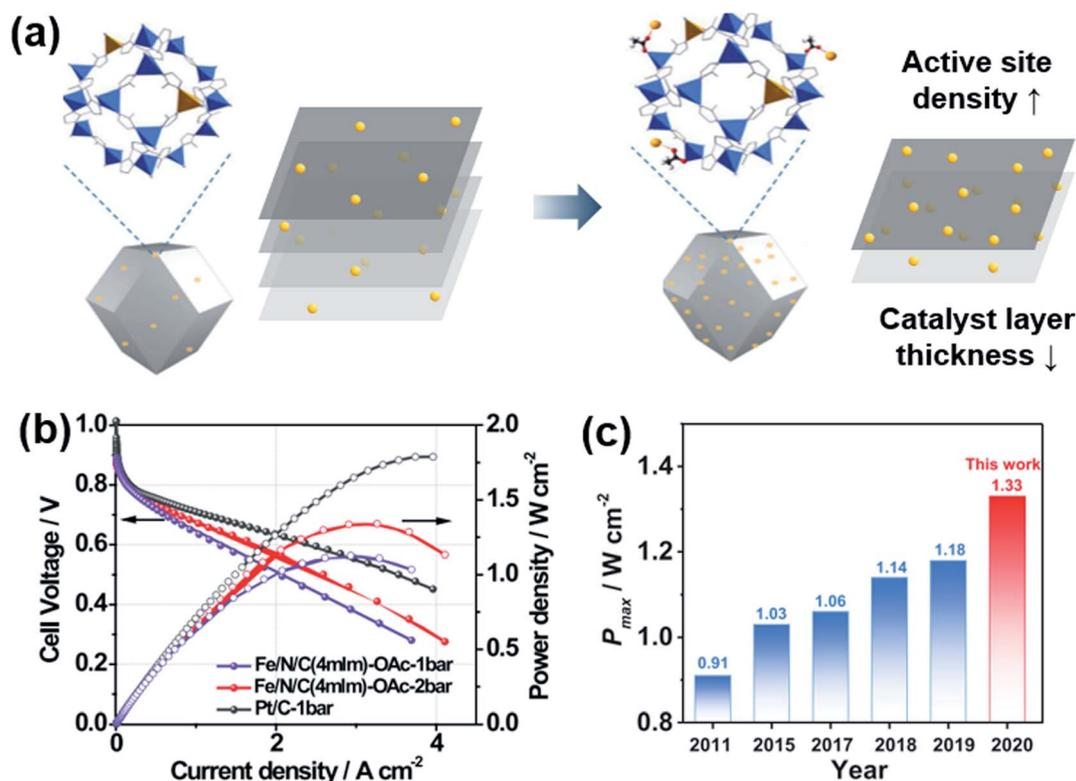
Fig. 7 (a) Schematic diagram of Fe-doping on ZIF-8 with acetates (OAc<sup>-</sup>). (b) Polarization and power density curves of Fe/N/C and Pt/C under H<sub>2</sub>/O<sub>2</sub> flow with 1 or 2 bar of backpressure. (c) Maximum power density ( $P_{max}$ ) of Fe-N-C catalysts in recent years. Reproduced from ref. 112 with permission, copyright 2021, Wiley-VCH.
