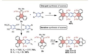
Scheme 4 Synthesis of acenes via the multiple addition of stannoles to benzynes. Reagents and conditions: (i) aryne (0.5 equiv.),  $^n$ BuLi (1.1 equiv.), toluene, 23 °C; (ii) aryne (1.1 equiv.),  $[nBu_4N][Ph_3SiF_2]$  (3 equiv.), DMAD (1.5 equiv.), toluene, 60 °C; (iii) aryne (2 equiv.),  $^n$ BuLi (1.1 equiv.), toluene, 23 °C.
