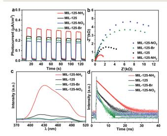
Fig. 3 (a) Photocurrent responses, (b) EIS Nyquist plots, (c) photoluminescence (PL) spectra (excited at 250 nm), and (d) time resolved PL spectra for MIL-125 and MIL-125-X ( $X = NH_2$ ,  $NO_2$ , Br) in MeCN.
