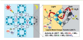
Scheme 1 Illustration showing the dark photocatalysis over MIL-125 and MIL-125 with different functional groups, MIL-125-X (X =  $NH_2$ ,  $NO_2$ , Br).
